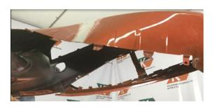
**K-BOND** body filler **applied to** bumper then twisted. It resists cracking without problems.
